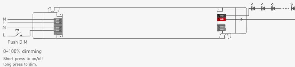
Dimming interface priority: First 0-10V, next Push DIM.
