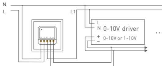
\* An external high-power relay switch is needed when total load current of the dimmer switch is more than 5A or inrush current is more than 50A/0.1S. The damaged dimmer switch resulting from overload current is not recovered by warranty.
